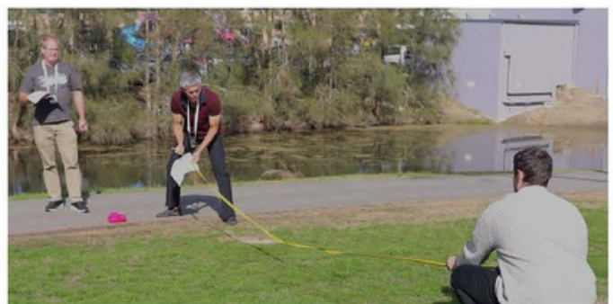
Robert Boland, Jason Chan and Zane van den Berg using similar triangles to calculate the width of a lake.
